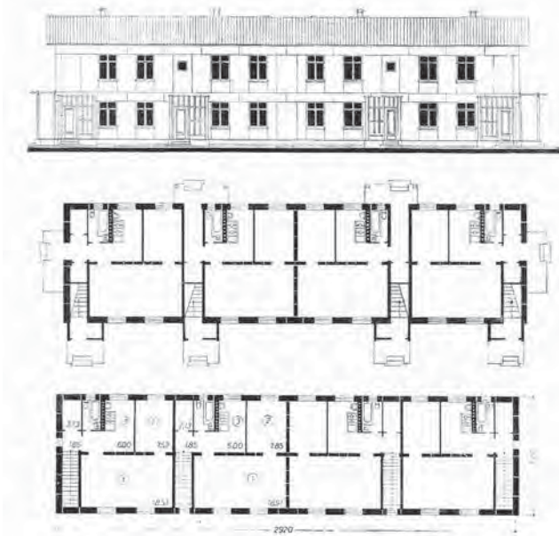
TWO-STOREY HOUSE FOR 8 APARTMENTS. GIPROGRAZHDANPROMSTROY DESIGN ORGANIZATION. SERIES 994 (RESIDENTIAL HOUSES USING CANE-FIBRE AND RUBBLE), 1958
