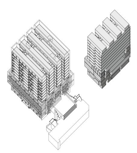
AXONOMETRIC VIEW AND AXONOMETRIC SECTION: RELATIONSHIP OF PUBLIC-ACCESSIBLE SPACES (LOWER STOREYS) AND ARCHIVE WITH OPERATIONAL SPACE INACCESSIBLE TO PUBLIC (UPPER STOREYS): VERTICAL PULSING CLUSTER
